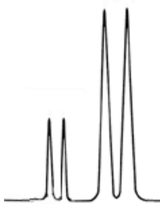
(b) ratio 1:1:3:3 Long range coupling of the CH 3 O protons with the CH is very small (close to zero). The essence of the question is to indicate the peak ratio's.
